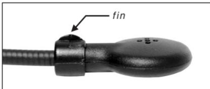
When installing the boom microphone included in the “Universal Microphone Kit”, place the velcro end of the boom microphone between the internal helmet cheek pad and the internal wall of the helmet shell. The boom microphone should be mounted so it is facing close to your mouth when you wear the helmet. You can use the enclosed velcro pad and holder for the boom microphone to ensure secure placement.
