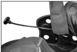
In the case of the wired microphone also included in the “Universal Microphone Kit”, attach the enclosed velcro pad for wired microphone to the inside of the chin guard for full-face helmets. Place the wired microphone on the velcro pad and connect it to the connector of the clamp unit.
