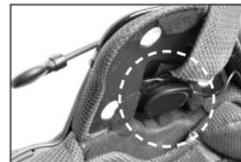
4. If you have any problem to clamp the speaker-microphone unit on the helmet for any reason, you may use the glued surface mounting adapter to attach the speaker-microphone clamp unit on the external surface of the helmet.
