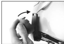
6. To remove the main headset from the speaker-microphone clamp unit, hold the lower part of the speaker-microphone clamp unit with your thumb and gently press down the hook on the upper part of the headset main unit with your index finger until it clicks out. You may have to do this to charge up or to carry the headset main unit.
