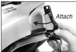
Sena recommends the clamp unit over the glued surface mounting adapter. Even though the glued surface mounting adapter is provided for convenience, Sena does not assume
