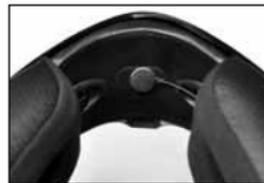
3. Place the helmet speakers along with the velcro pads, centered to your ear, in the ear pockets of the helmet. If the helmet has deep ear pockets, you can use the speaker pads to place the speakers closer to your ears.
