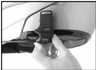
2. Please adjust the direction of the microphone so that the **triangular mark** on the microphone is pointing towards your mouth. The **fin side** of the microphone should be facing outward; away from your lips.
